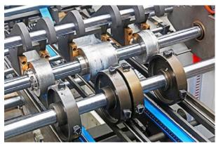
5. Every part of forming and collecting system can be adjusted according to the size of mold. The whole collection system can be opened to change mold and install the forming parts conveniently.
